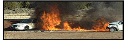
Image 7 – Trail of fire from leaking fuel
