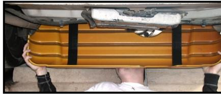
Image 9 – FIRE Panel raised onto fuel tank
