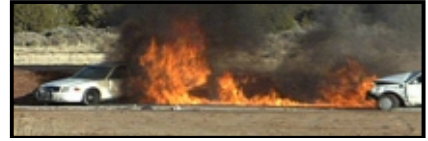
Image 7 – Trail of fire from leaking fuel
