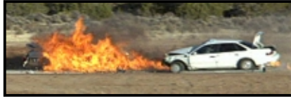
Image 6 – Fireball forms around the CVPI
