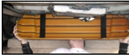
Image 9 – FIRE Panel raised onto fuel tank
