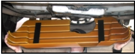
Image 8 – FIRE Panel installation
