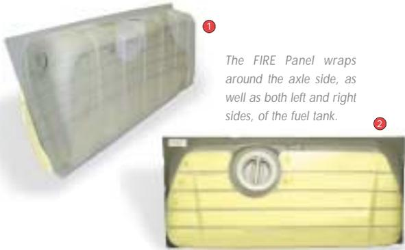
The FIRE Panel wraps around the axle side, as well as both left and right sides, of the fuel tank.
